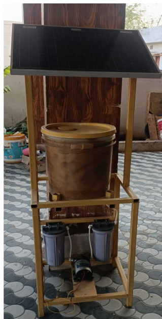
Figure 2 : Model of water based purification system
