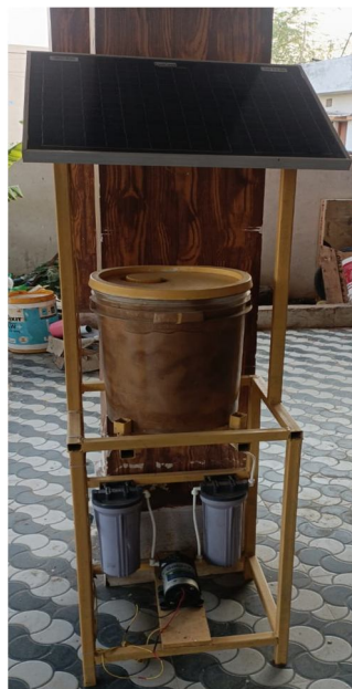
Figure 2 : Model of water based purification system
