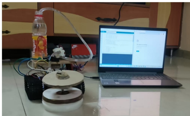
Fig.4 (B) Working Prototype of Solar Panel cleaning robot
