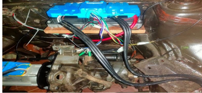
Figure 2. Motor and motor controller
