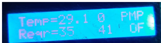
Fig.5: Temperature is displayed on LCD
