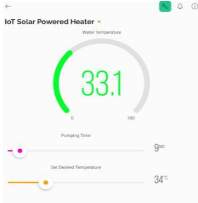
Fig.4. Controlling of the system (pumping time and set desired temperature) through Blynk app
