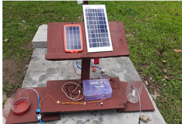
Fig.3. Solar Water Heater using an IoT
