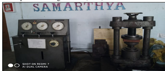
Fig. 13: Compression testing machine
