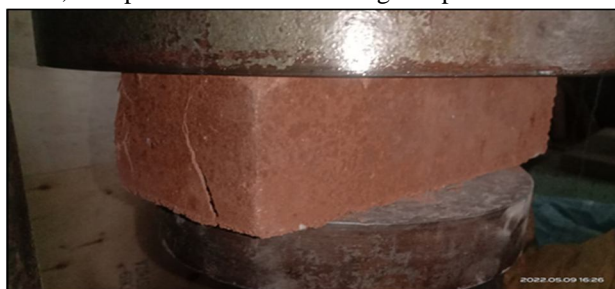
Fig. 15: Failure of brick
