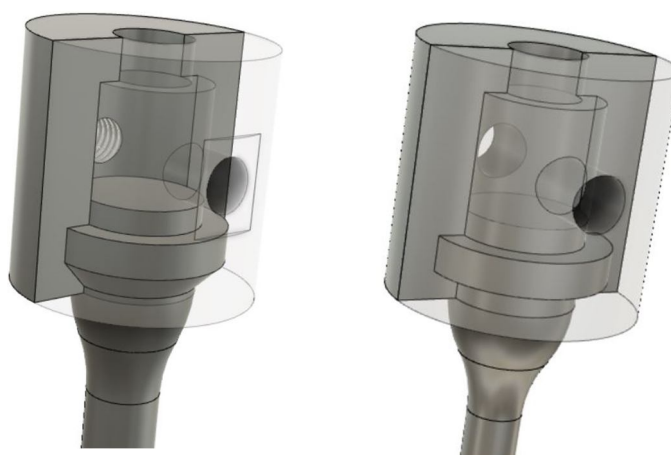
Fig. 7- Rendering of designed grips to the new sample geometry.
