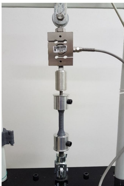
Fig. 10- A Specimen placed in the tensile testing machine.
