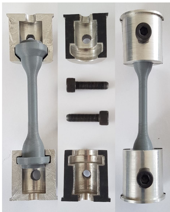
Fig. 8- Grips specially designed for the new sample geometry.
