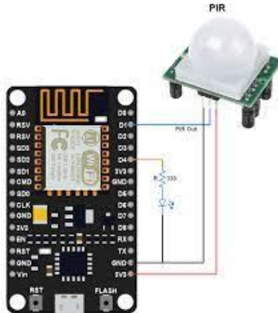
Fig. 1. Circuit diagram of the PIR circuit interfaced
