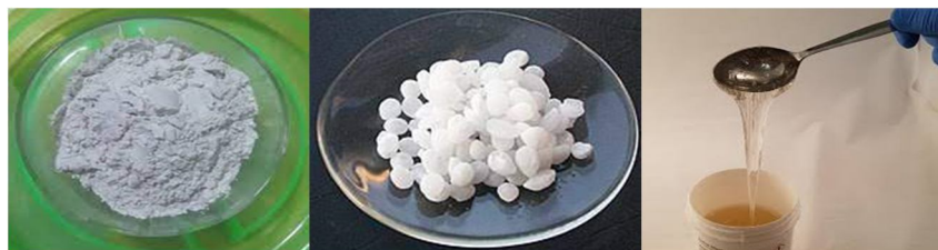
Fig 1: Materials used in this study GGBS – Sodium Hydroxide Pellets - Sodium Silicate
