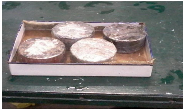
Figure 4.5 Sorptivity test on GPC
