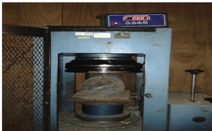
Figure 4.2 Test setup of split tensile strength
