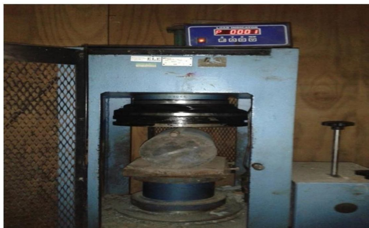
Figure 4.2 Test setup of split tensile strength
