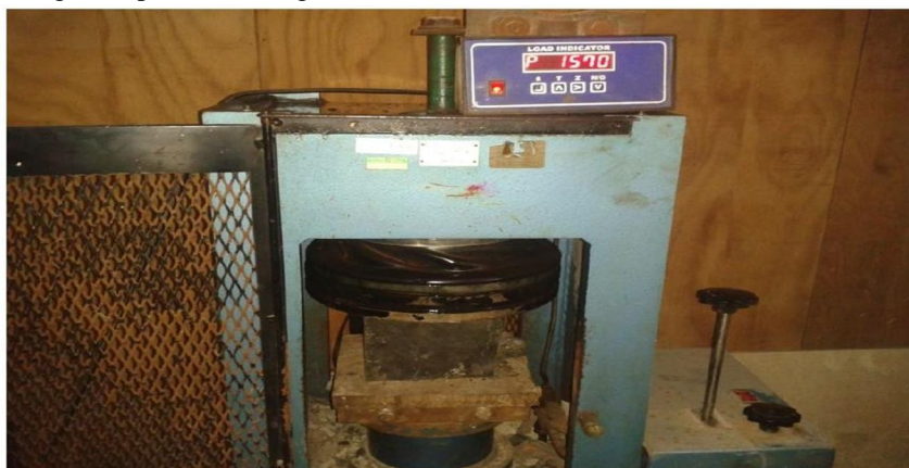
Figure 4.1 Test setup of compressive strength
