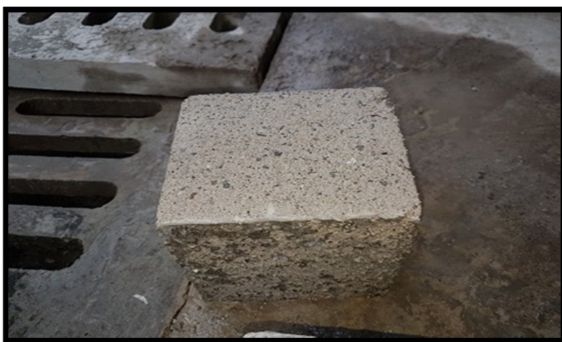
Photo 2- Showing effect of alkaline NaOH solution on concrete cube
