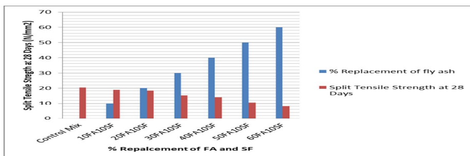
Fig 4.2.2: Graphical Arrangement of Split Tensile Strength at 28 Days (N/mm 2 )
