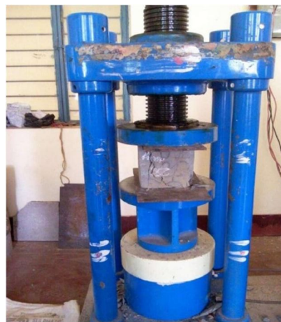
Fig. 5 Compression Testing Machine
