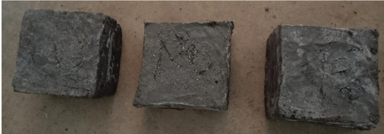
Fig. 5: PET Bottle Reinforced Concrete Cube Blocks
