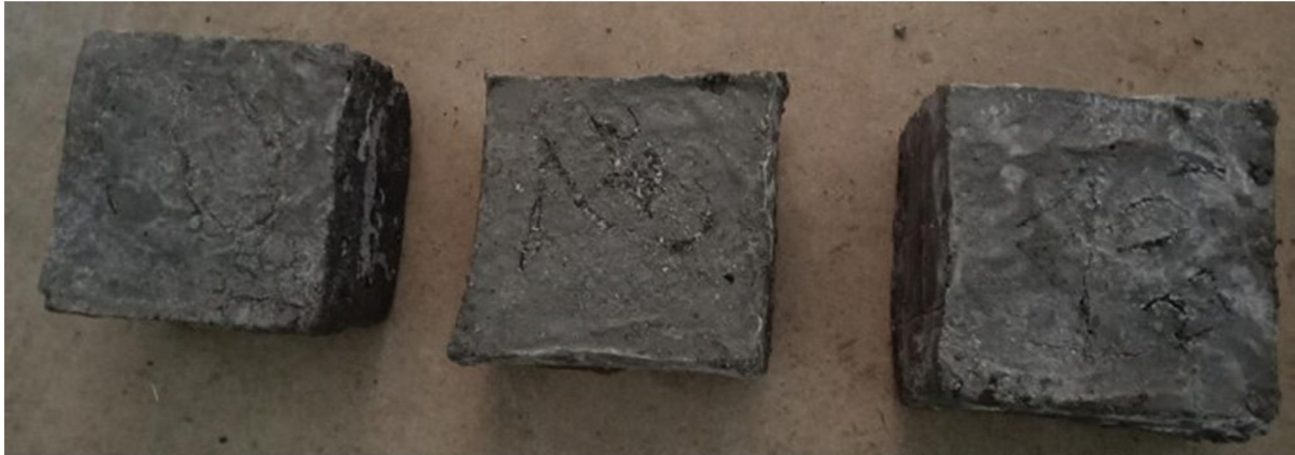
Fig. 5: PET Bottle Reinforced Concrete Cube Blocks
