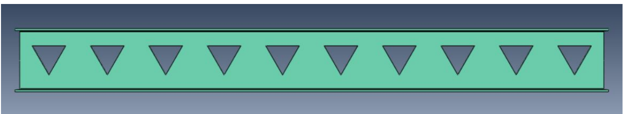
Fig. 2 Castellated beam with Triangular opening
