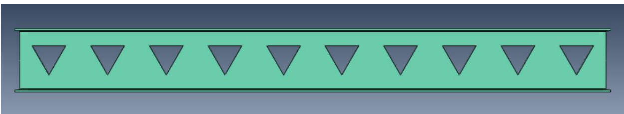
Fig. 2 Castellated beam with Triangular opening
