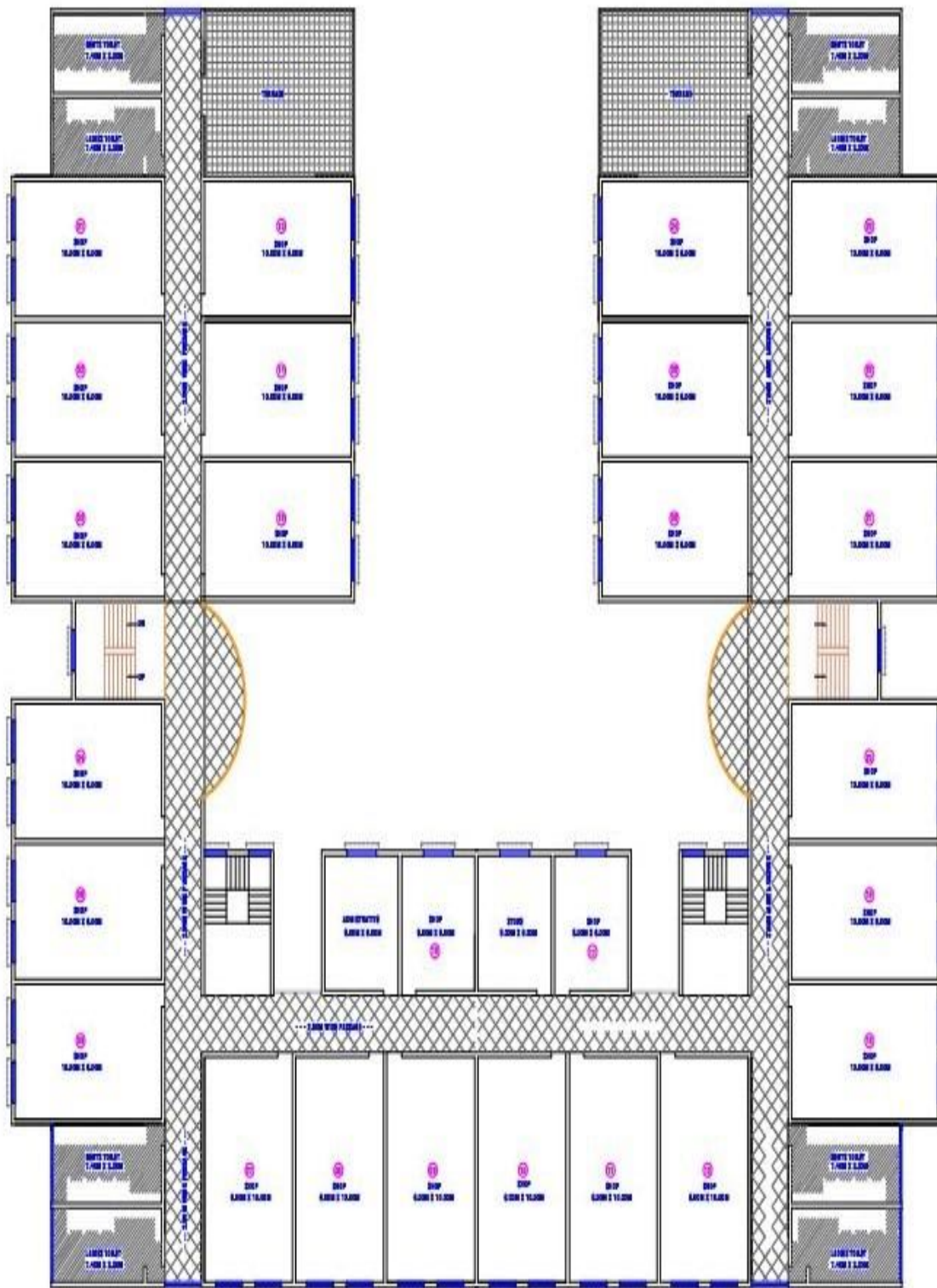
Fig 1 Typical C-Shape Floor Plan (Modelled in AutoCAD)
