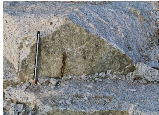
FIG7: sericitization which result in greenish colour.
