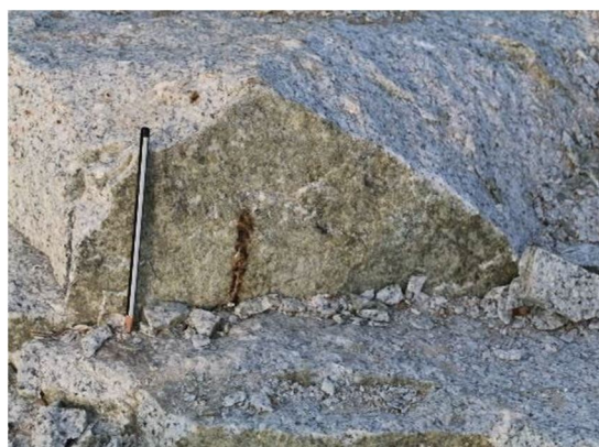
FIG7: sericitization which result in greenish colour.
