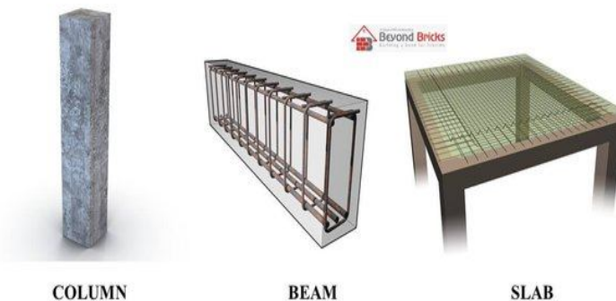
Fig 10. Example of Building Elements
