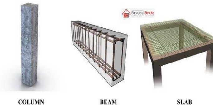
Fig 10. Example of Building Elements
