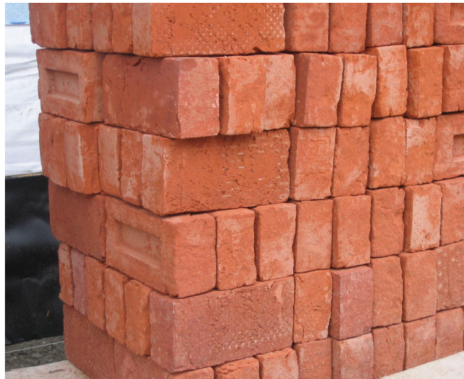
Fig 4a. Fired Bricks
