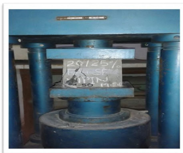
Fig 2.1: Compressive strength test procedure and loading condition
