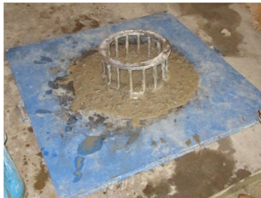
Fig 3.8 J-Ring flow for reference mix SCC
