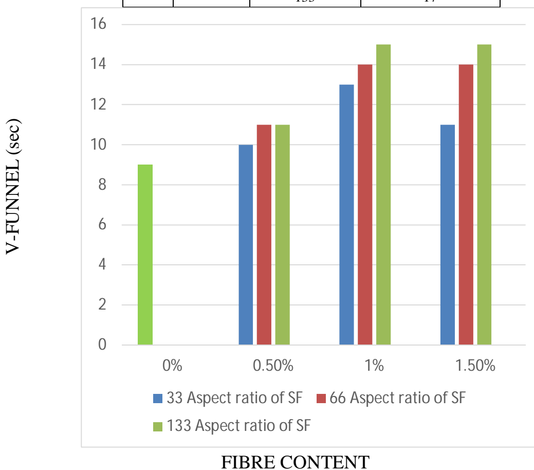
Fig 4.6: V-Funnel flow of SFRSCC with increase in fibre content & various Aspect ratios
