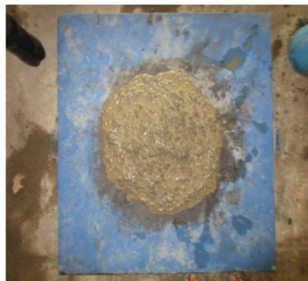
Fig 4.5 Slump flow for 1.5% fibre content SCC
