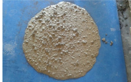
Fig 4.3 Slump flow for 0.5% fibre content SCC
