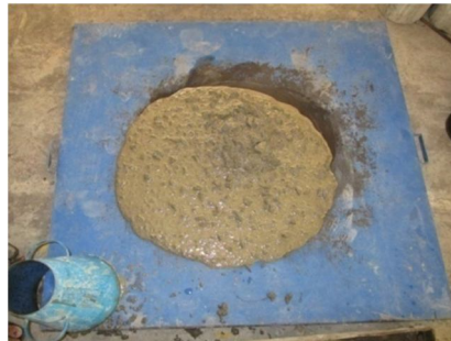
Fig 4.4 Slump flow for 1% fibre content SCC
