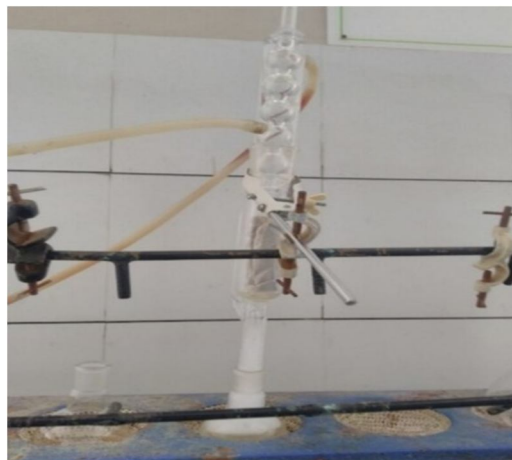
Fig-3 Soxhlet extraction process
