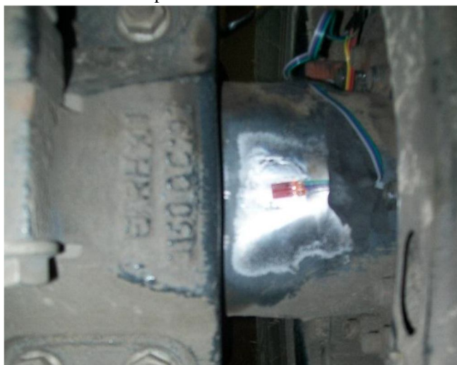
Fig. 2 Strain gauge pasted on axle bottom
