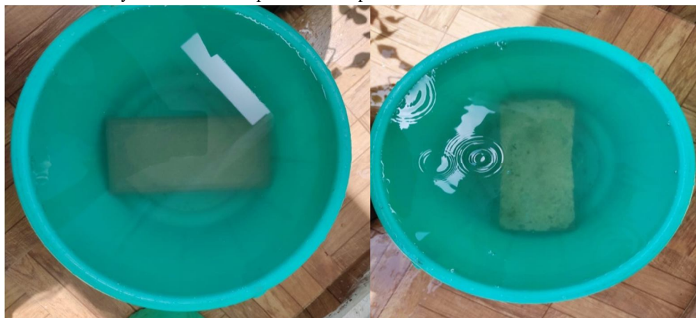
Fig. 3: Water Absorption Test
