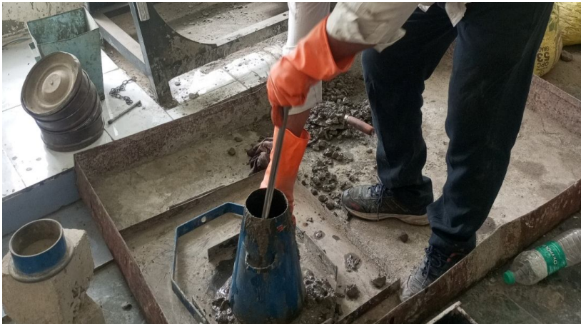
Fig. 5 Filling of Slump Cone in 3 Layers (Each layer has 25 Times Tamping with 16mm Bar)
