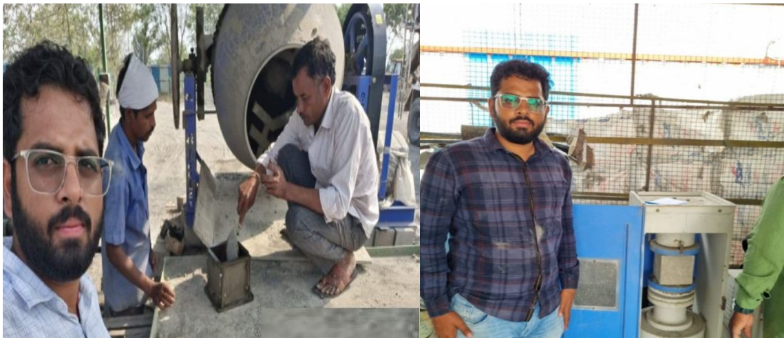
Fig. 7 Glass fiber reinforced Concrete Cube casting for experimentation
