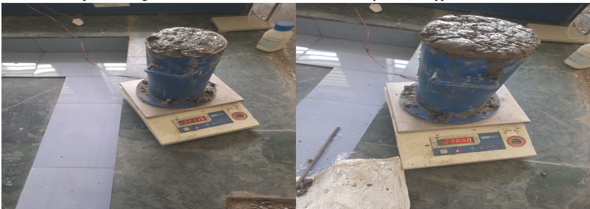
Fig. 6 wt. of partially and fully compacted concrete
