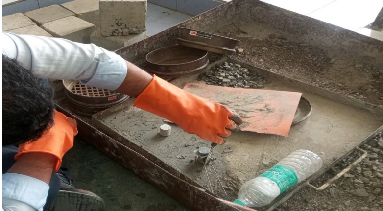
Fig. 4 Mould of Le Chatelier Apparatus is Filled with Cement Paste
