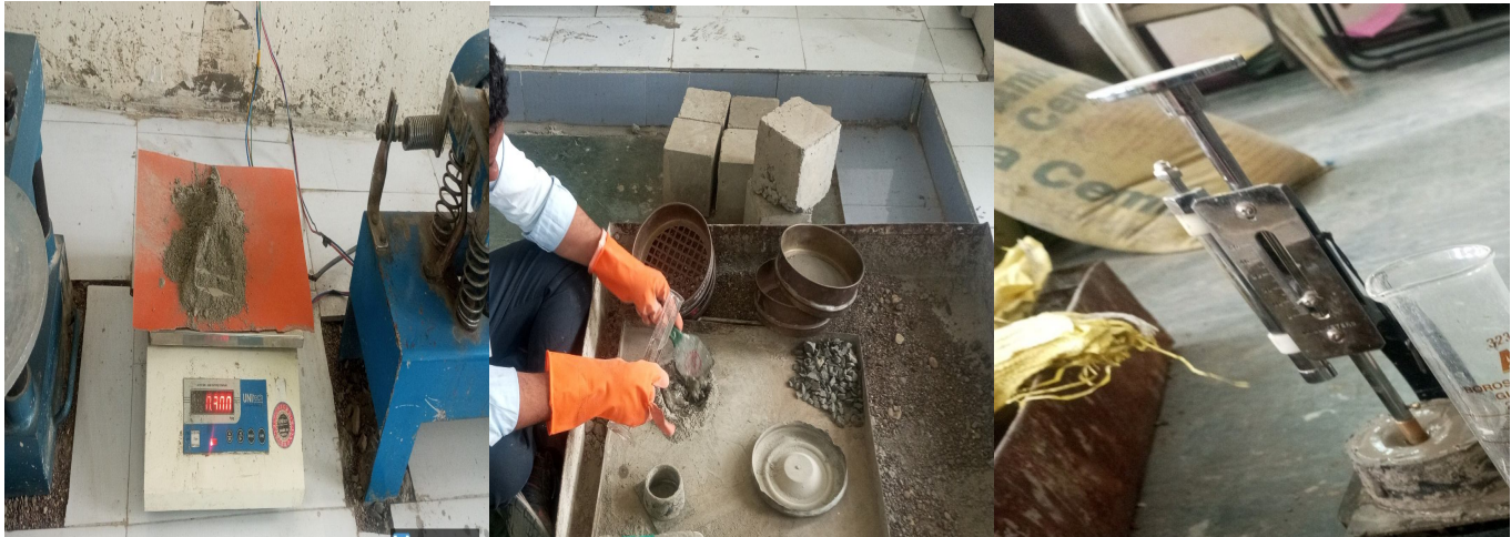
Fig. 2 Testing of Normal Consistency of Cement
