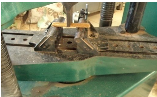
Fig. 8 Experimental setup used for bending test.
