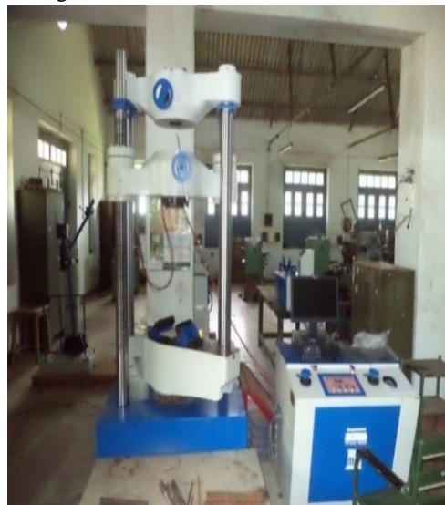
Fig. 7 Computerized universal testing machine.
