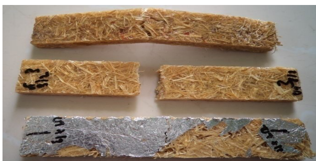
Fig. 9 Bending test specimen after test is done.
