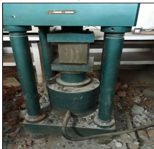
Fig 8: Compressive Strength Testing machine
