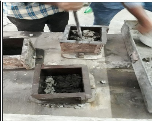
Fig 5: Preparation of Cubes
