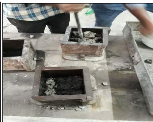
Fig 5: Preparation of Cubes
