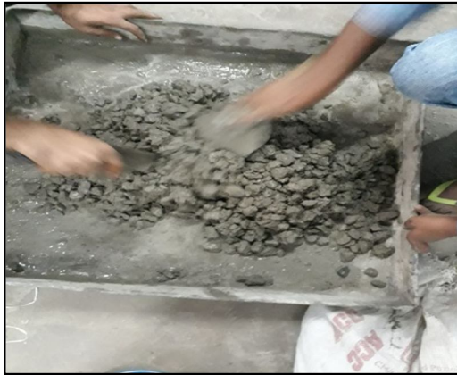
Fig 4: Mixing of Aggregates
