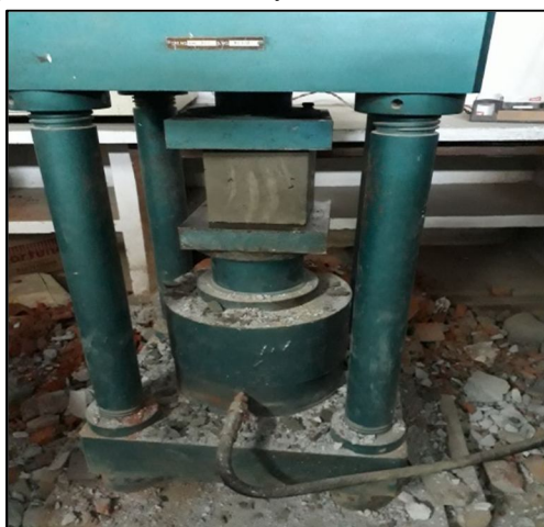
Fig 8: Compressive Strength Testing machine
