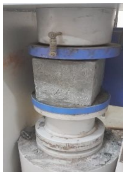
Figure 5: Testing on Cubes Figure 6: Cube casting
