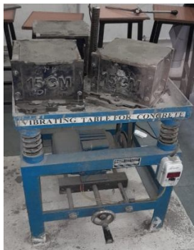
Figure 5: Testing on Cubes Figure 6: Cube casting
