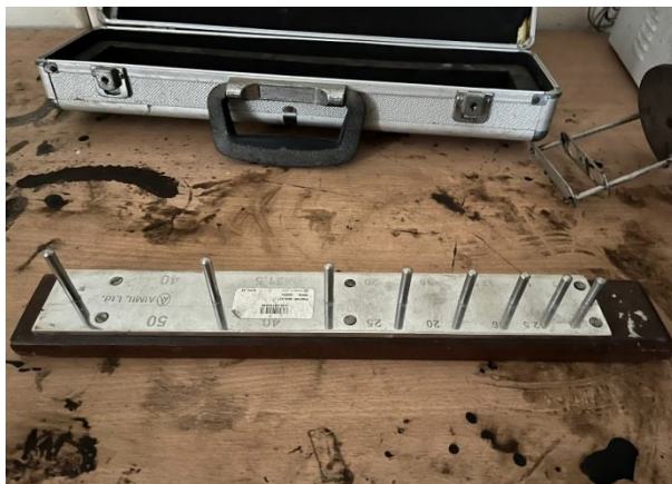
Fig 3.11 Flakiness Index Apparatus
