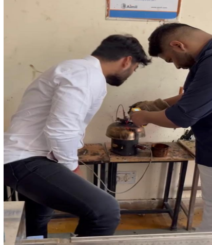
Fig 3.4 Pensky Martin Apparatus
