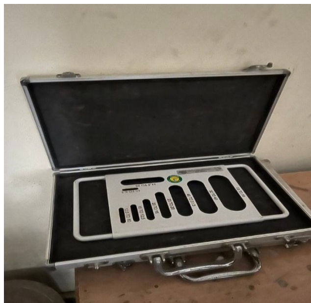
Fig 3.13 Elongation Index Apparatus
