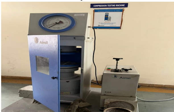
Fig3.6 Compression Testing Machine
