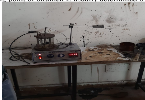
Fig 3.5 Ring And Ball Apparatus
