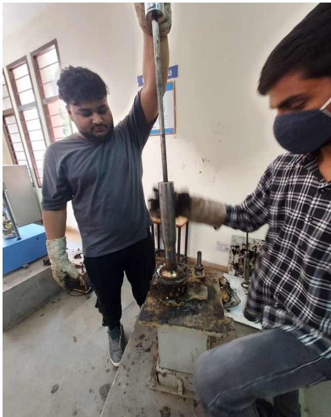
Fig 3.14 Performing Marshall Stability Test
