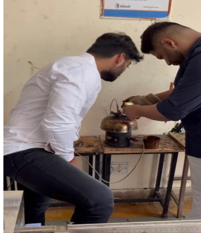
Fig 3.4 Pensky Martin Apparatus
