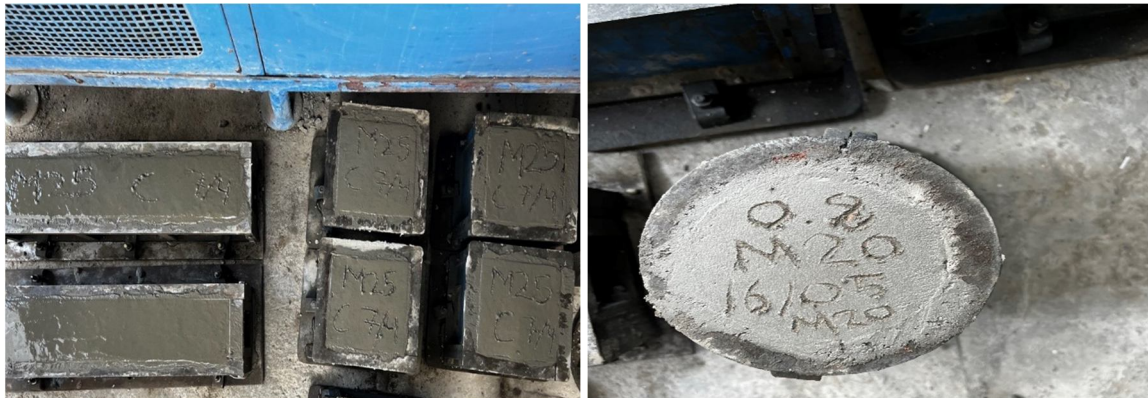
Fig. 1: Specimens of Self Curing Concrete
