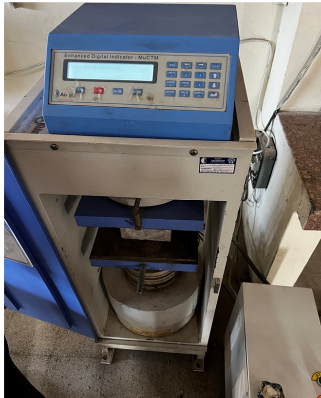
Fig. 2: Testing of Self Curing Concrete
