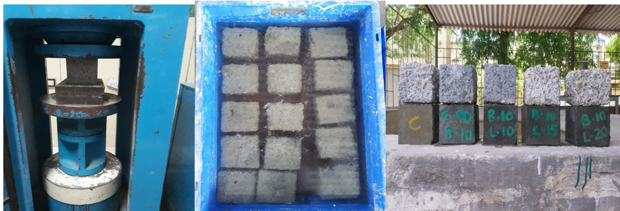
Fig. 6. Durability tests conducted on the ternary concrete – Acid resistance test
