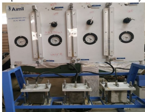
Fig. 5. Durability tests conducted on the ternary concrete – Water impermeability test
