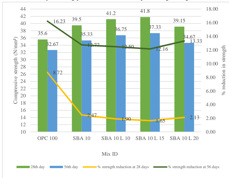
Fig. 13. The compression strength and percentage of strength loss at the 28 th and 56 th days of Na 2 SO 4 curing
