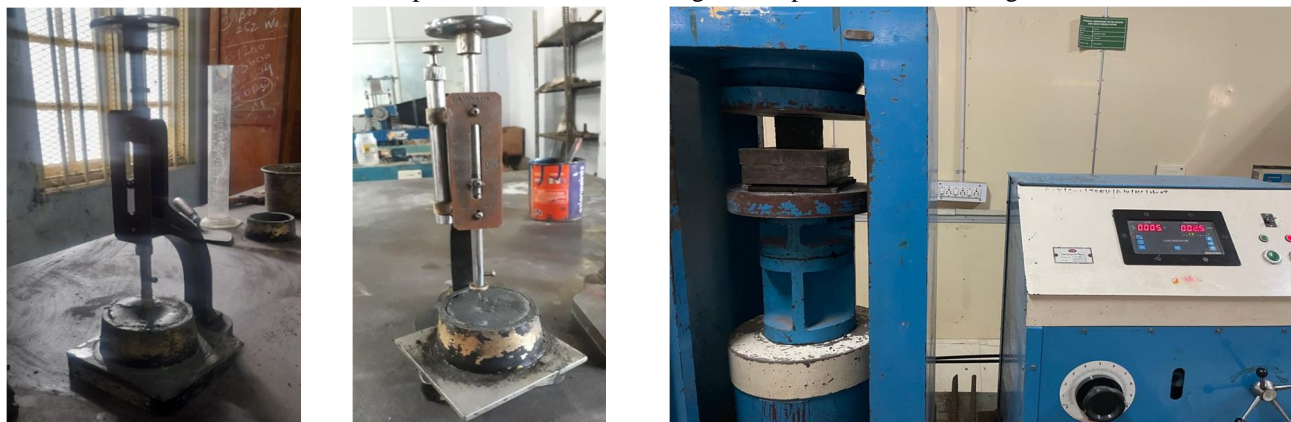
Fig. 1. Standard Consistency Test, Initial setting time Test and Compression Test
