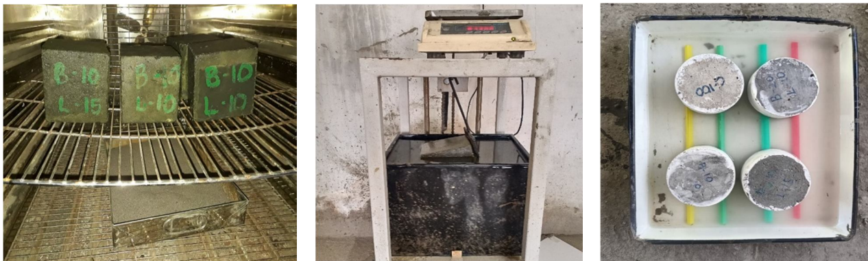
Fig. 4. Durability tests conducted on the ternary concrete – Water absorption test, Porosity test, Sorptivity test
