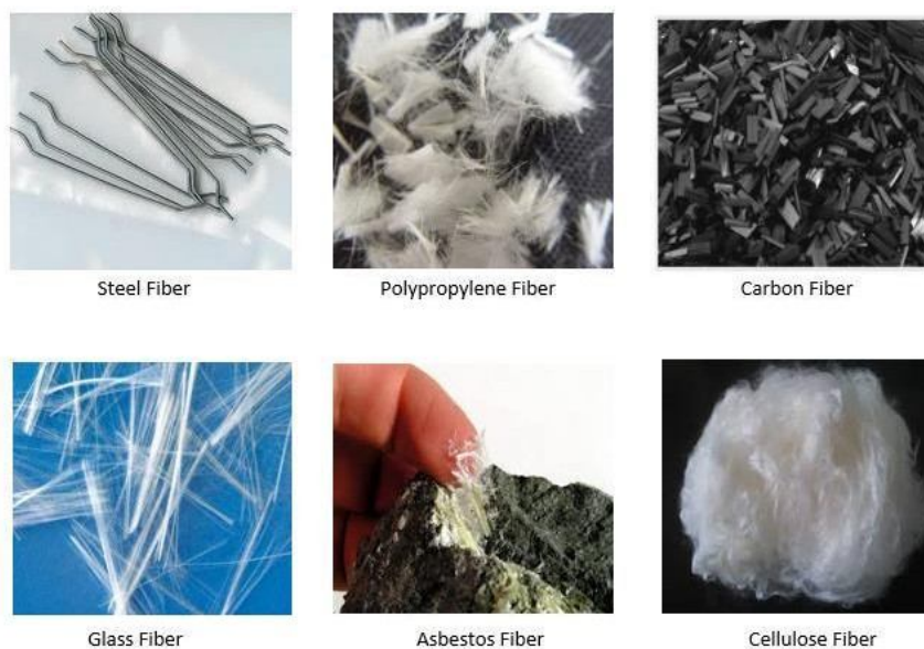
Fig. 2 Types of fiber reinforcement
