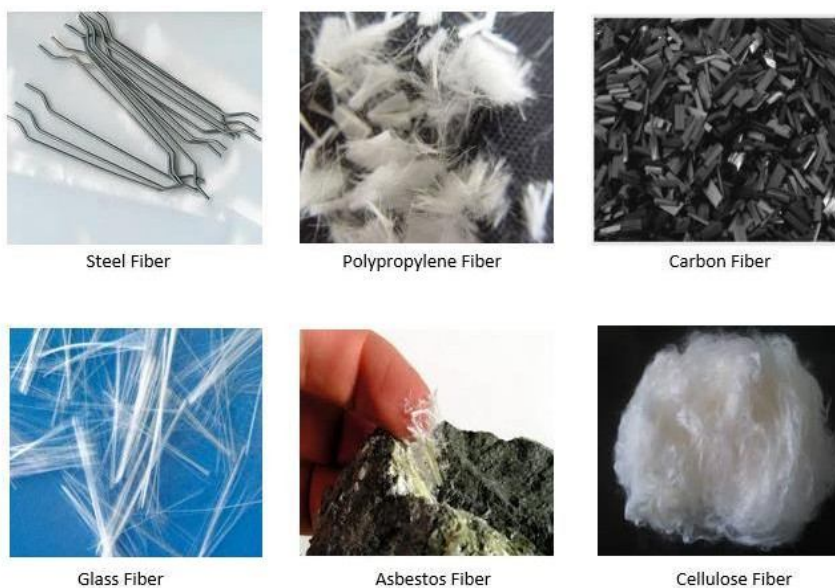
Fig. 2 Types of fiber reinforcement
