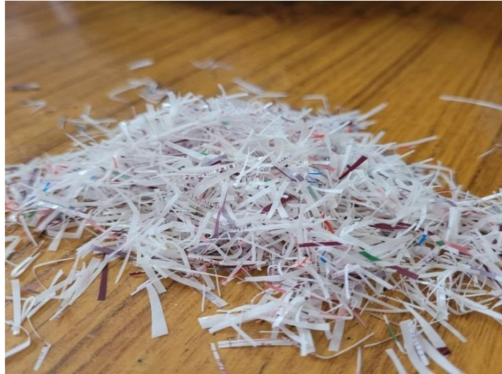
Fig. 3 Shredded milk packets
