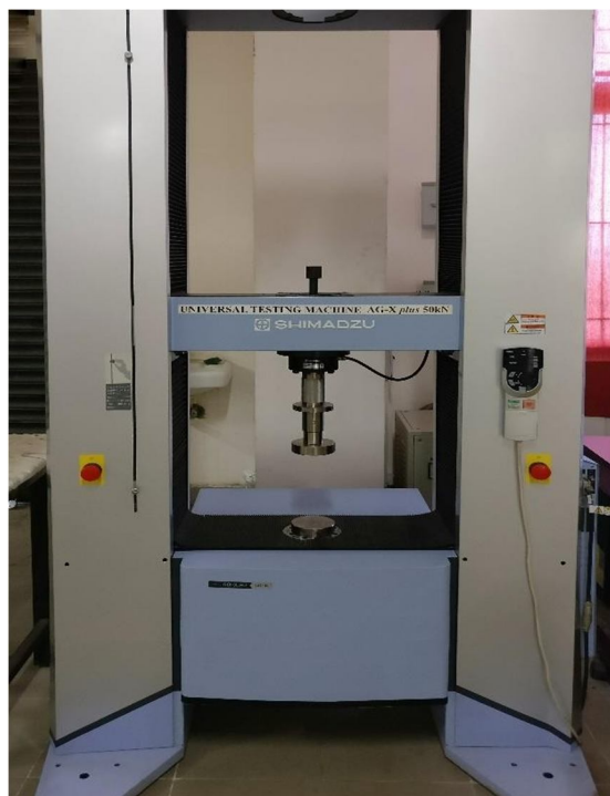
Fig 4.4 Universal testing machine apparatus
