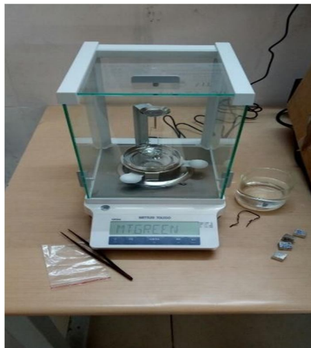
Fig 4.1 Density measurement apparatus
