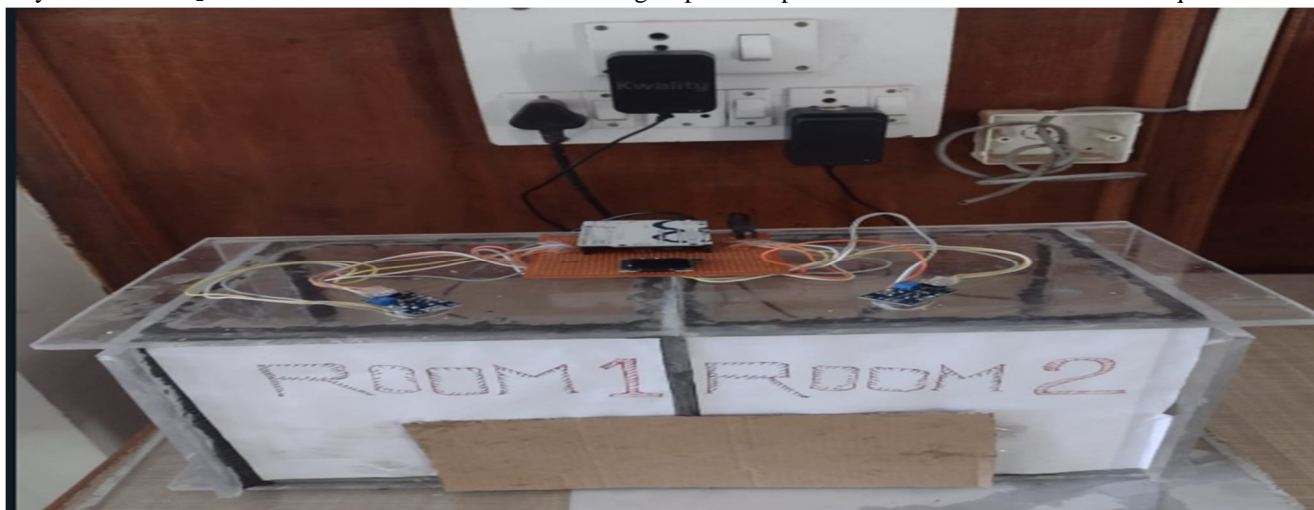
Fig.4 Carbon sequestration study chamber with MQ 135 sensors
