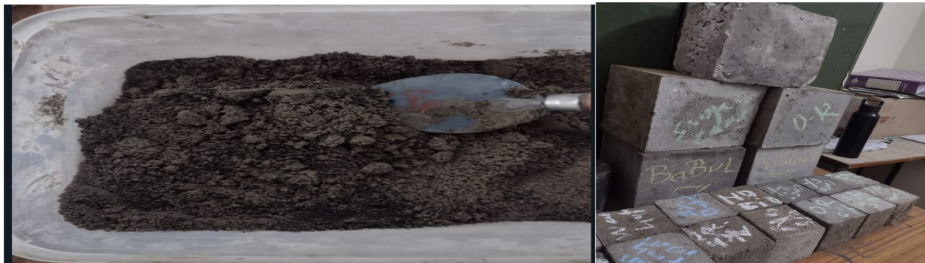
Fig.3 mortar cubes and concrete cube after Sugarcane Bagasse biochar enrichment
