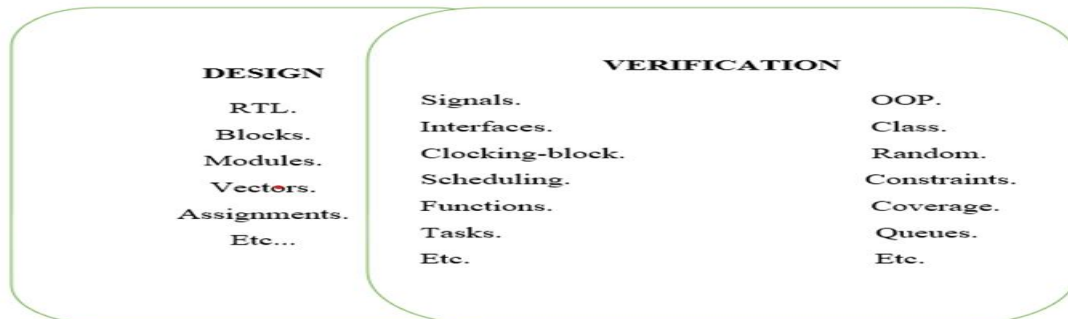
Fig 1 Components of Design and Verification [1]
