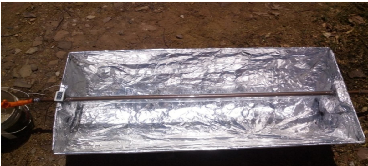
Figure 4 Parabolic trough collector developed has aluminum foil as reflector copper tube without plane glass cover
