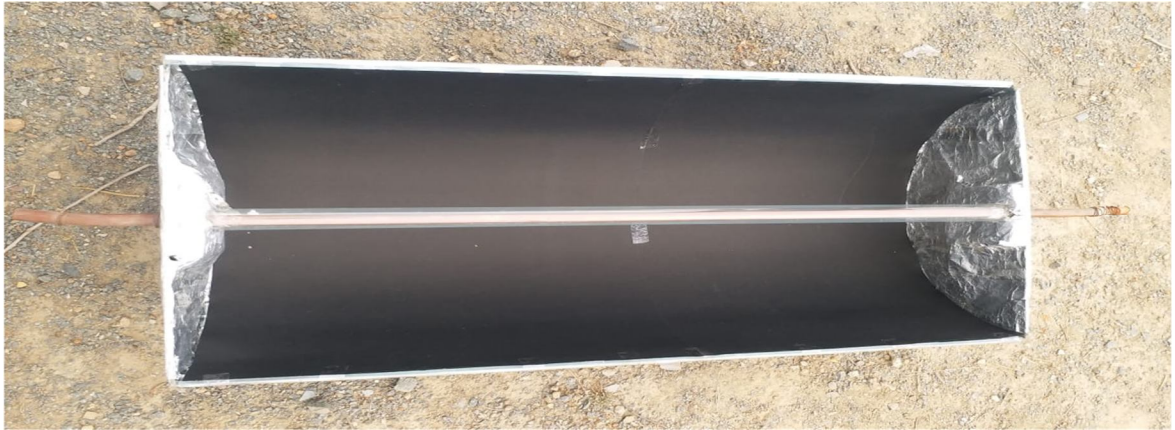
Figure 2 Parabolic trough has black carbon material foil.
