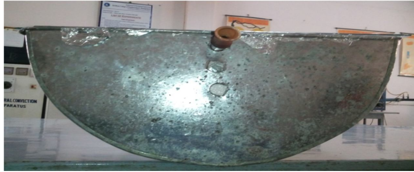
Figure 9 Side view of parabolic trough collector
