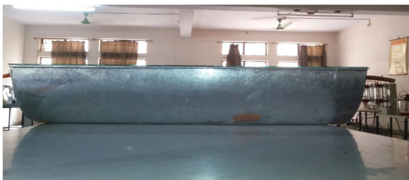
Figure 10 Front view of parabolic trough collector
