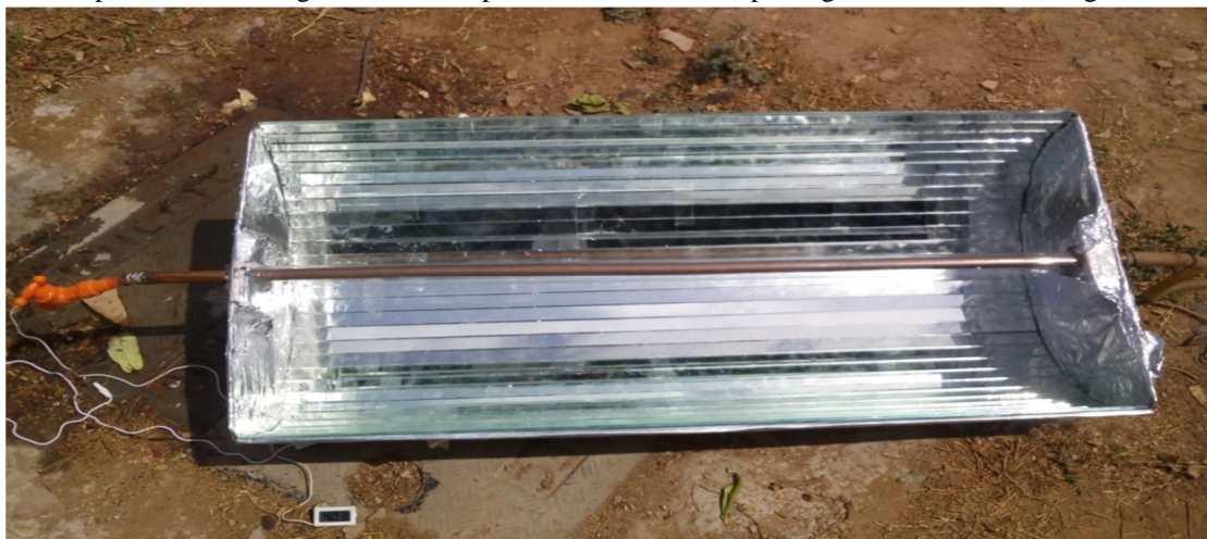
Figure 7 Parabolic trough collector has rectangular mirror strips, copper tube as reflector with plane glass cover
