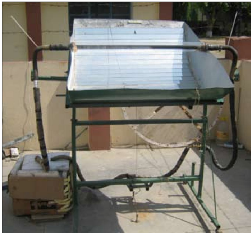
Figure 13 Experiment taken for black carbon foil as reflector with and without plane glass cover on face
