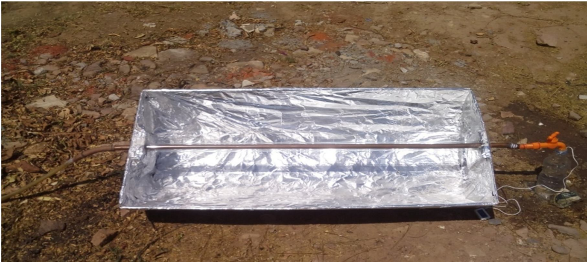
Figure 5 Parabolic trough collector developed has aluminum foil as reflector, copper tube with plane glass cover
