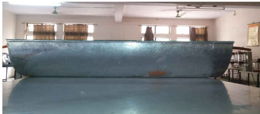
Figure 10 Front view of parabolic trough collector
