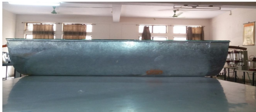
Figure 10 Front view of parabolic trough collector
