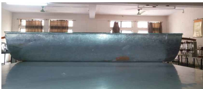
Figure 10 Front view of parabolic trough collector
