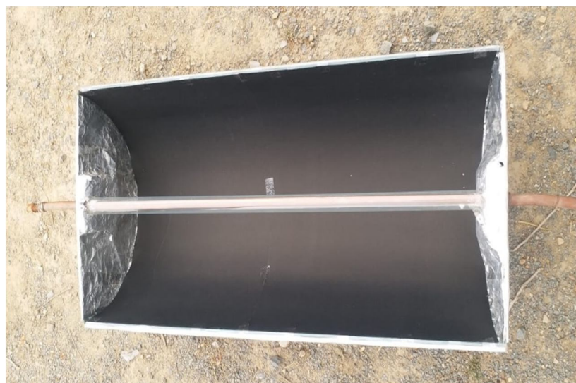
Figure 8 Top view of parabolic trough collector
