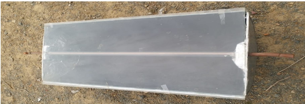
Figure 3 Parabolic trough has black carbon material foil with plane glass cover
