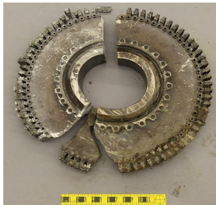
Figure 2: Burst fragments of turbine disc
