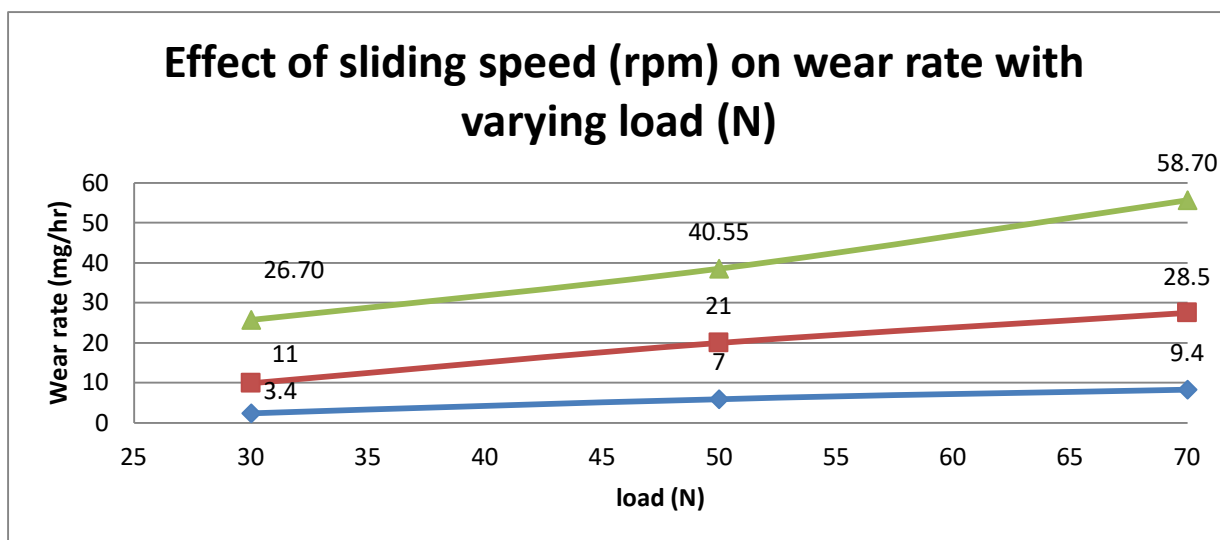
Fig 3: Effect of sliding speed (rpm) on wear rate with respect to varying load (N)
