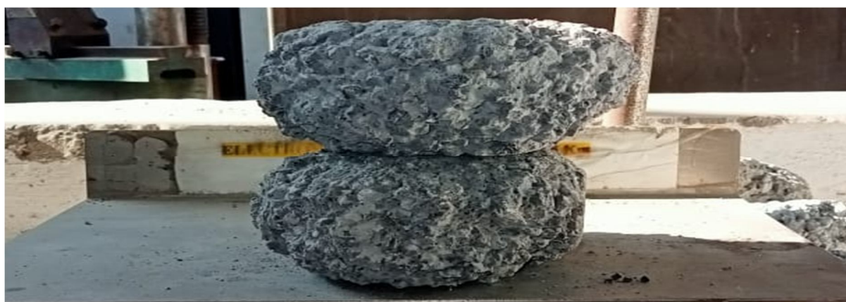
Image G pcpb after Cantabro abrasion
