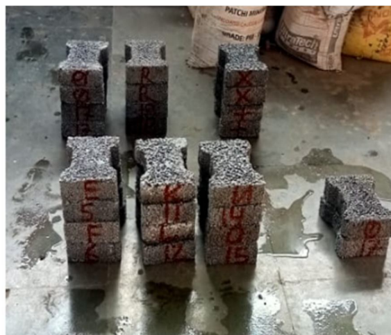
image E 28 days cured wet ppb
