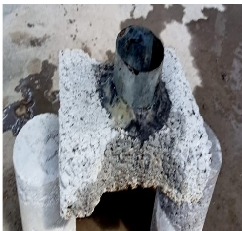
Image H plumber putty sealing ring bottom
