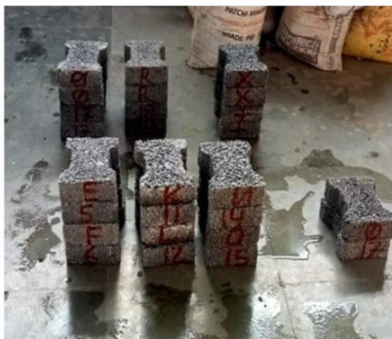
image E 28 days cured wet ppb
