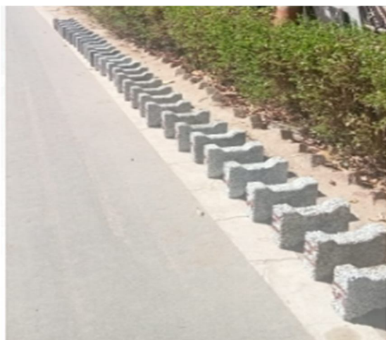
Image D ppb drying in sun light
