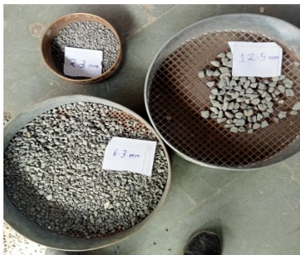
Image B sieve analysis of FA
