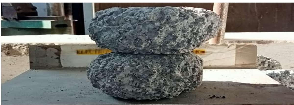
Image G pcpb after Cantabro abrasion
