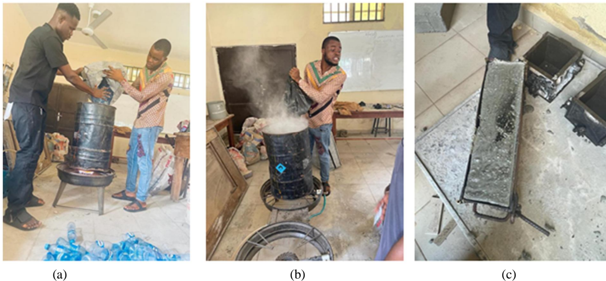
Figure 1: (a) melting of the plastic. (b) Mixing of melted plastic with fine aggregate. (c) After moulding the block
