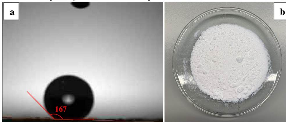
Fig 7. Silica aerogel material; a) contact angle of super hydrophobic silica aerogel, b) General image
