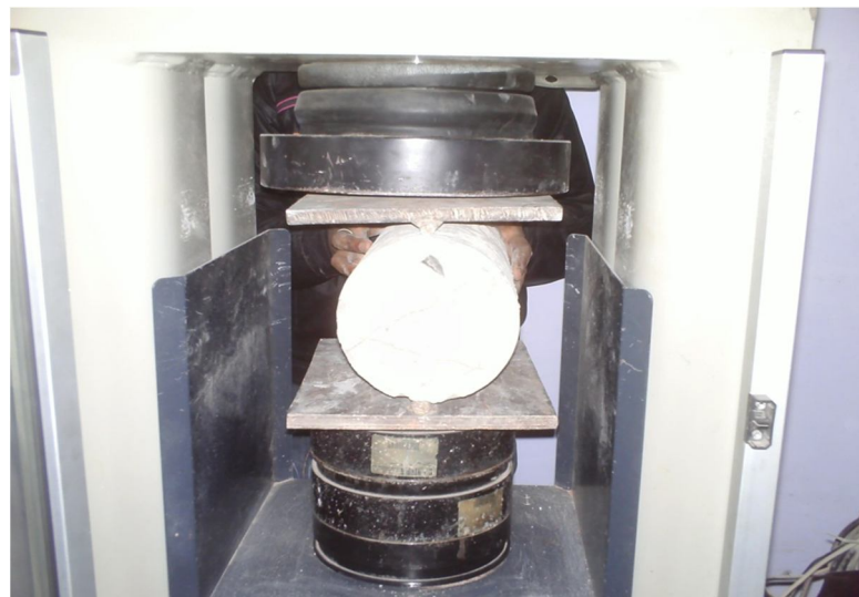
Fig 4 Split Tensile Testing
