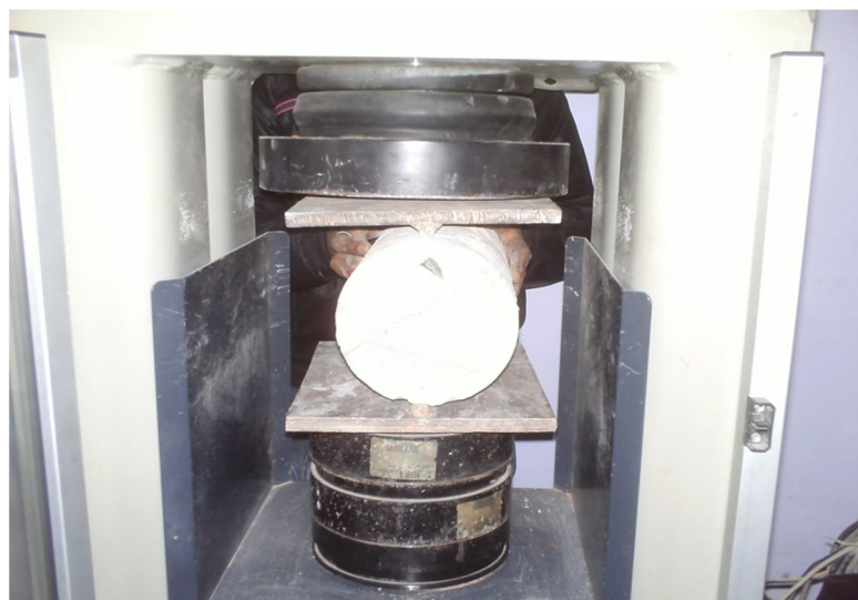
Fig 4 Split Tensile Testing
