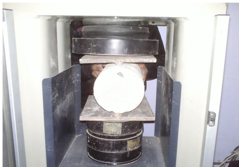
Fig 4 Split Tensile Testing
