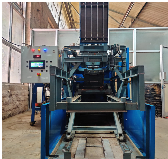
Fig 1: Roller Compactor cum Rut Analyser (RCRA)
