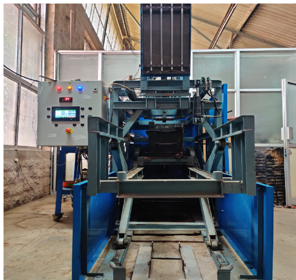
Fig 1: Roller Compactor cum Rut Analyser (RCRA)
