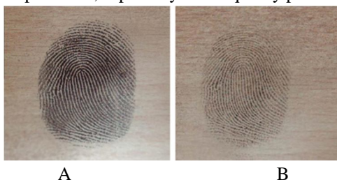
Fig 2: Fingerprints developed on polythene for the (A) first and (B) fifth impression in succession
