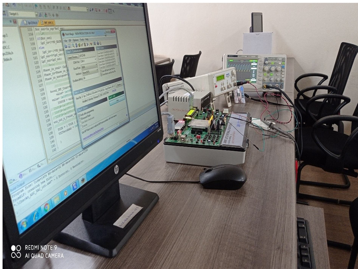
Fig. 12 Experimental Set-up: A linked setup with host connected to LPC2148 evaluation board which in-turn is connected to function generator for providing input and a DSO to view Input and output time domain waveform.
