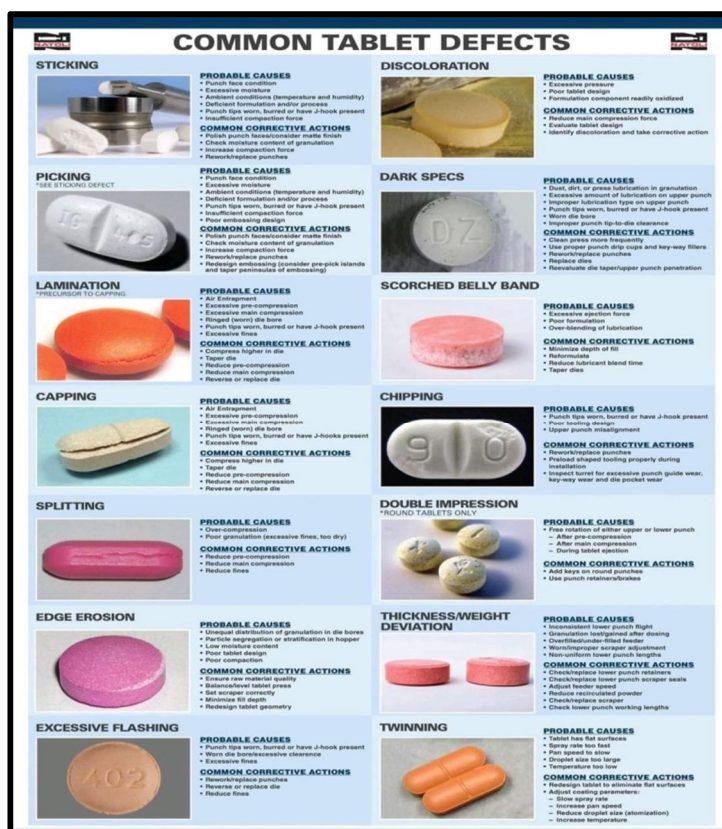
Fig.5 Defects of tablets [13]
