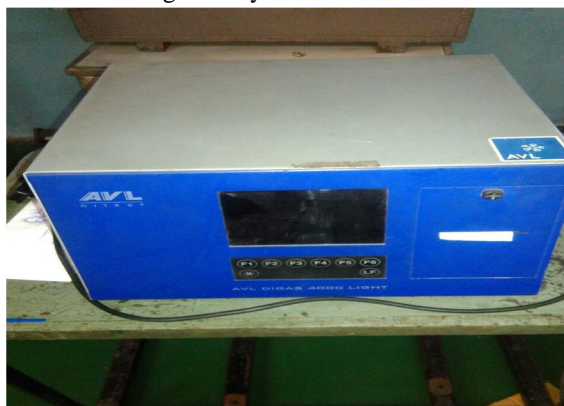
Figure 4.1 Photograph of AVL Di-gas 4000 gas analyzer
