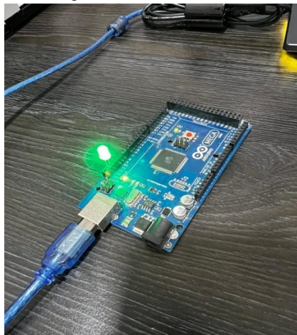
Fig. 5.5 Green LED simulates opening a barrier
