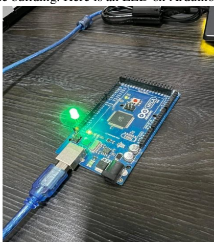
Fig. 5.5 Green LED simulates opening a barrier
