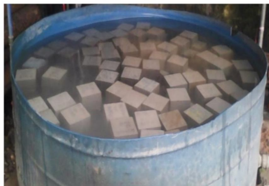
Figure 4: Cubes in Curing Tank
