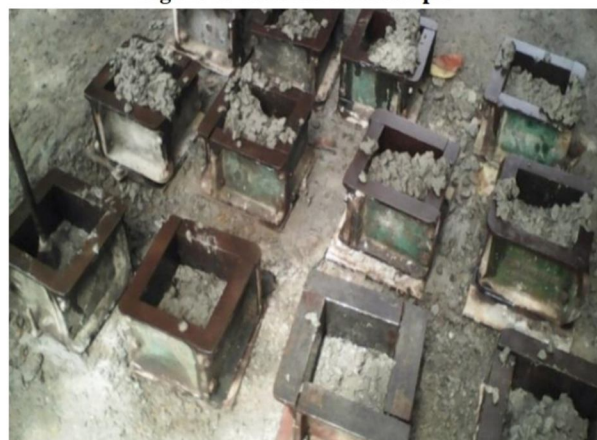
Figure 3: Concrete Placing in Cube Moulds
