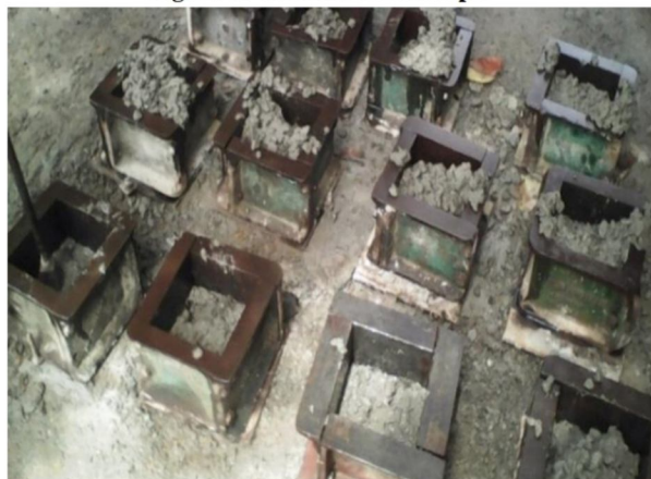
Figure 3: Concrete Placing in Cube Moulds
