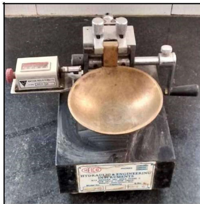
FIG 5.5: Liquid Limit Apparatus
