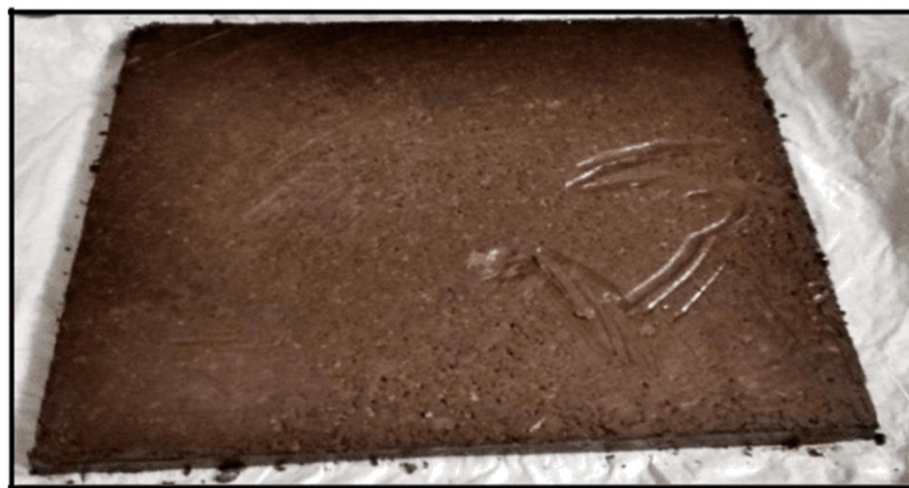
FIG 5.14: BC Soil Layer Compacted for PRE Determined Depth
