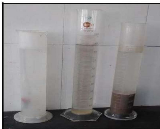
FIG 5.8: Final Stage Of Hydrometer Analysis After 24hrs.
