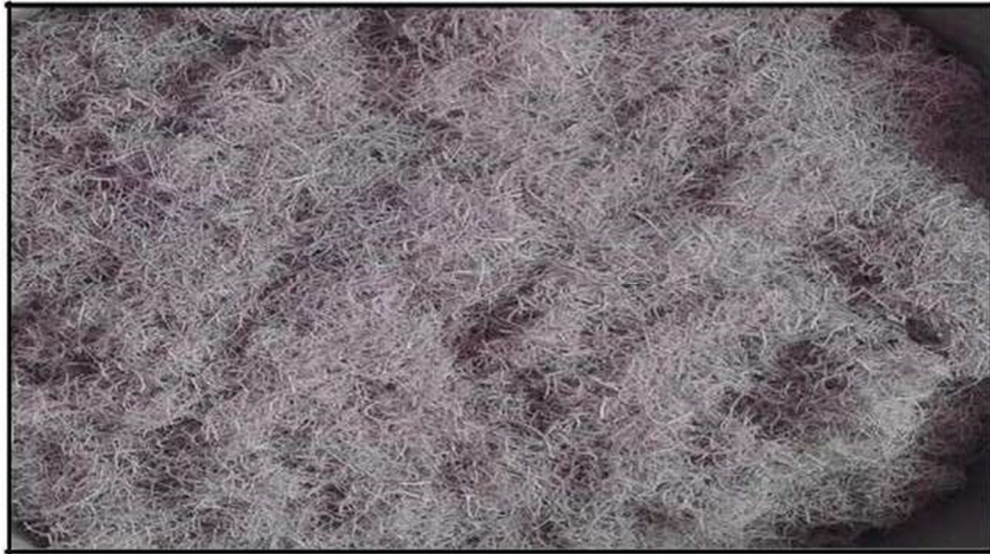
Fig 4.8: Final Treated Coir Fiber Obtained After All Treatment
