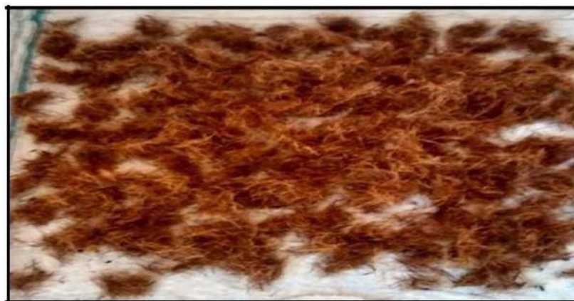
FIG 4.5: Drying After Washing With Distilled Water
