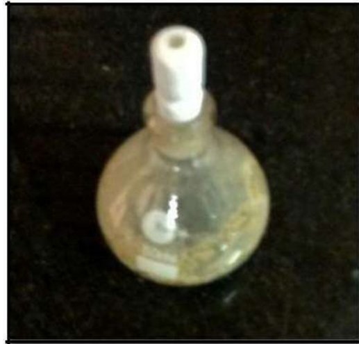
FIG 5.4: 50 ML Density Bottle ALONG With LID
