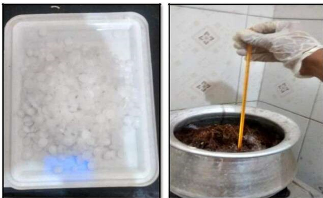
FIG 4.4: Treatment Of Detergent Scoured Cf Using NaohSolution
