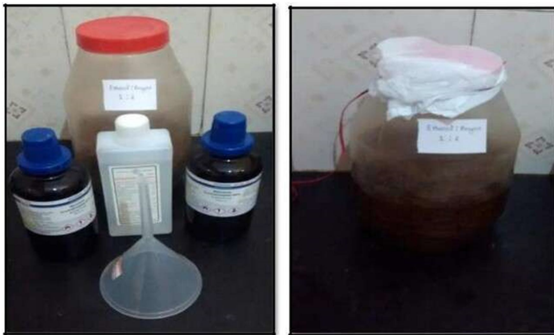
FIG 4.3: Immersion in Ethanol: Benzene (1:2)
