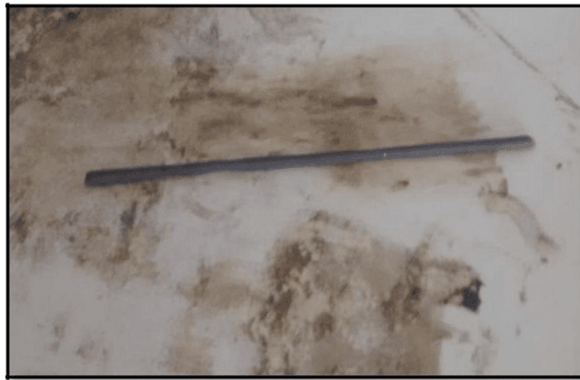
FIG 5.6: Plastic Limit Test
