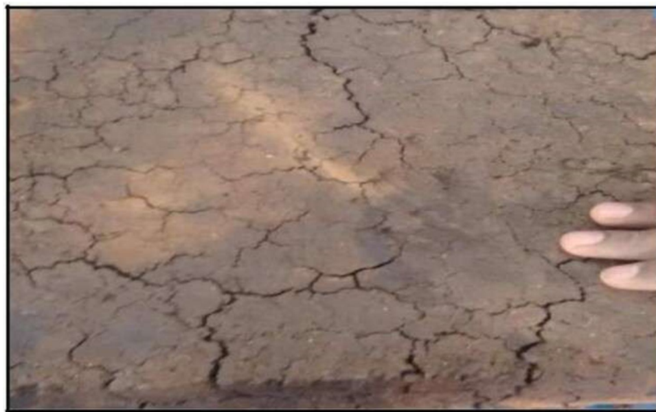
FIG 5.1: BC Soil Shrinkage Cracks after testing
