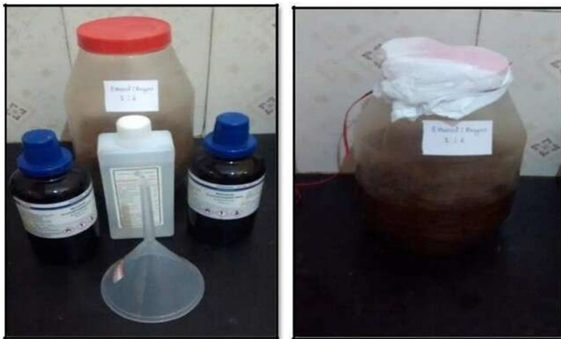
FIG 4.3: Immersion in Ethanol: Benzene (1:2)
