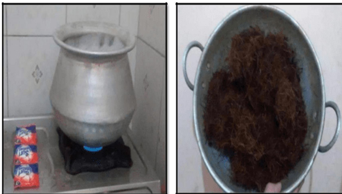
FIG 4.2: Treatment of CF With Detergent Solution & Washing With Distilled Water
