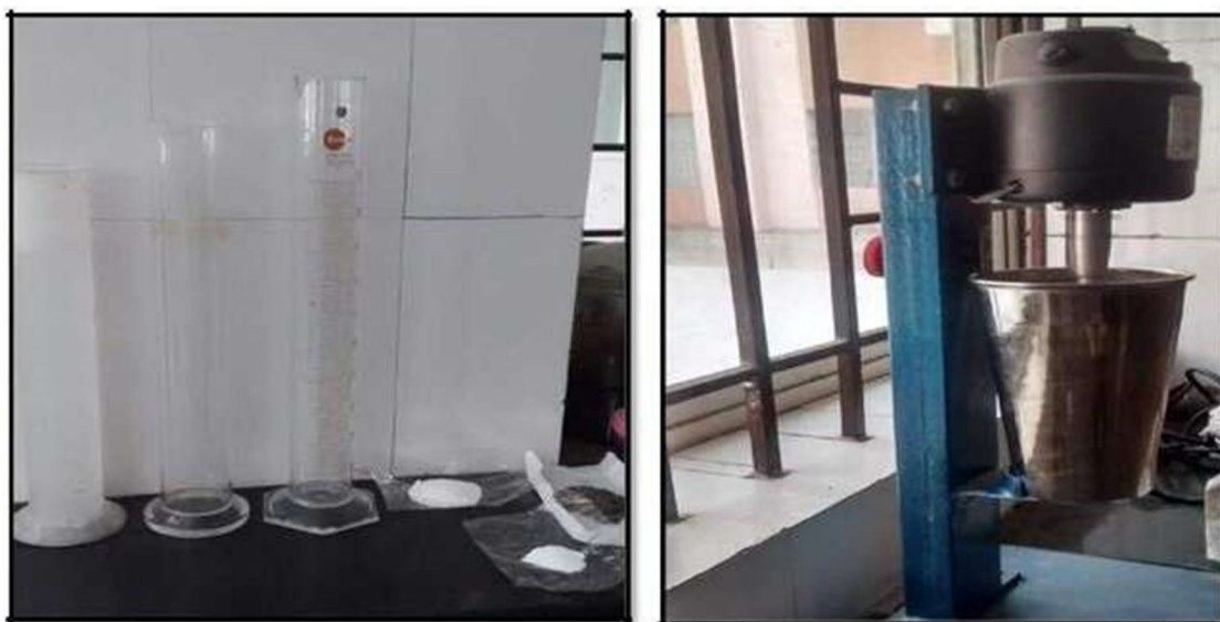
FIG 5.7: Initial Preparation During Hydrometeranalysis
