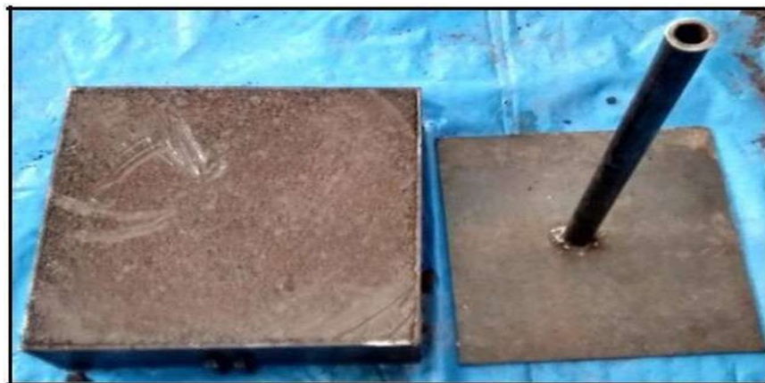
FIG 5.13: Steel Mould & Tamper Used For Preparing Bc Soil Layer
