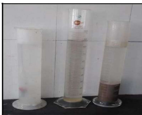
FIG 5.8: Final Stage Of Hydrometer Analysis After 24hrs.
