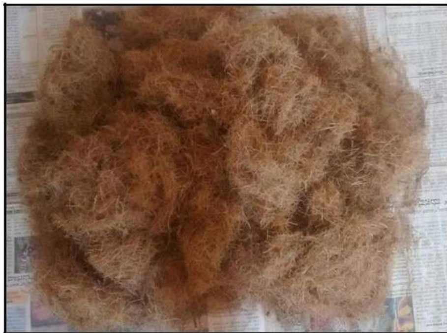
FIG 4.1: Coir Fibers Before Treatment
