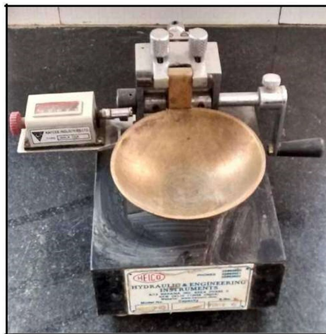
FIG 5.5: Liquid Limit Apparatus
