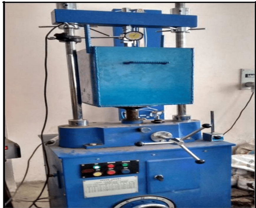
FIG 5.17: Model Footing Test Apparatus
