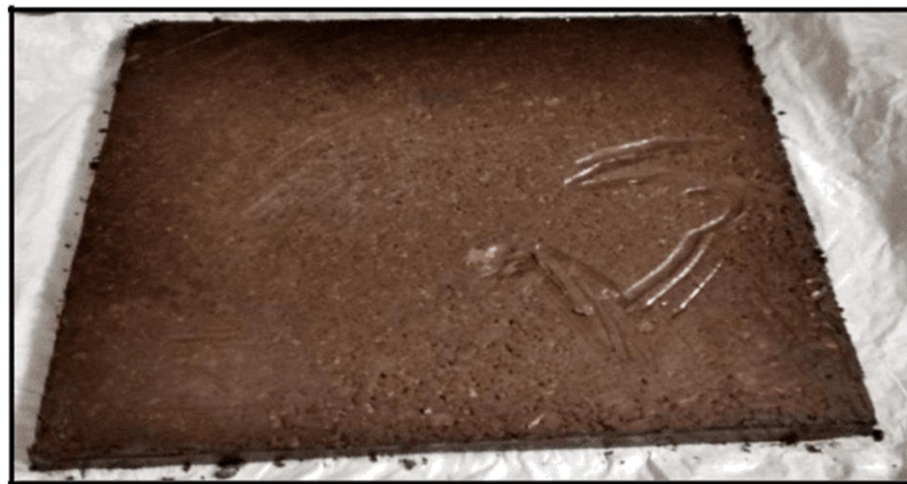
FIG 5.14: BC Soil Layer Compacted for PRE Determined Depth
