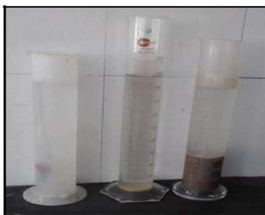
FIG 5.8: Final Stage Of Hydrometer Analysis After 24hrs.
