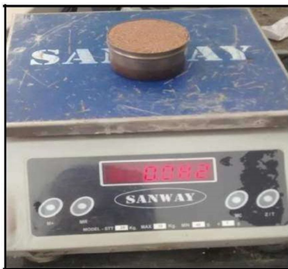
FIG 5.10: Determination Of Saw Dust density By Soil Raining Technique
