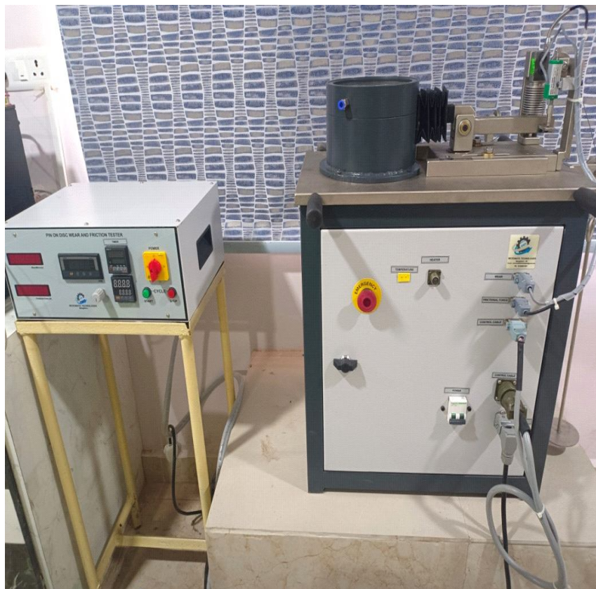
Fig.12. Experimental setup of Pin on disc wear testing Equipment
